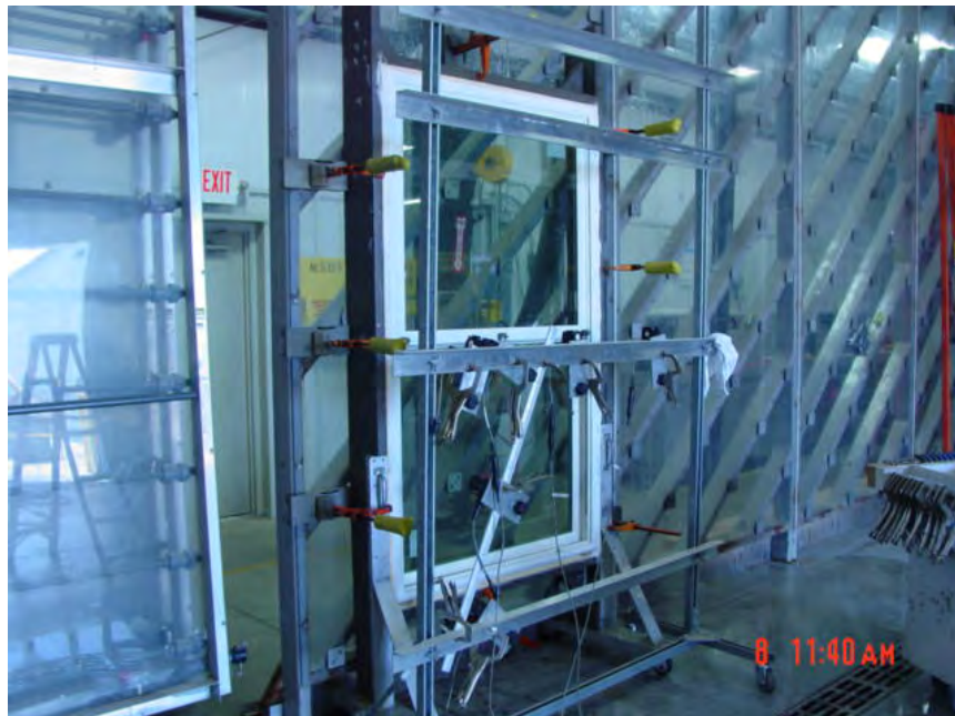
Photo #1 Structural loading of double hung.
