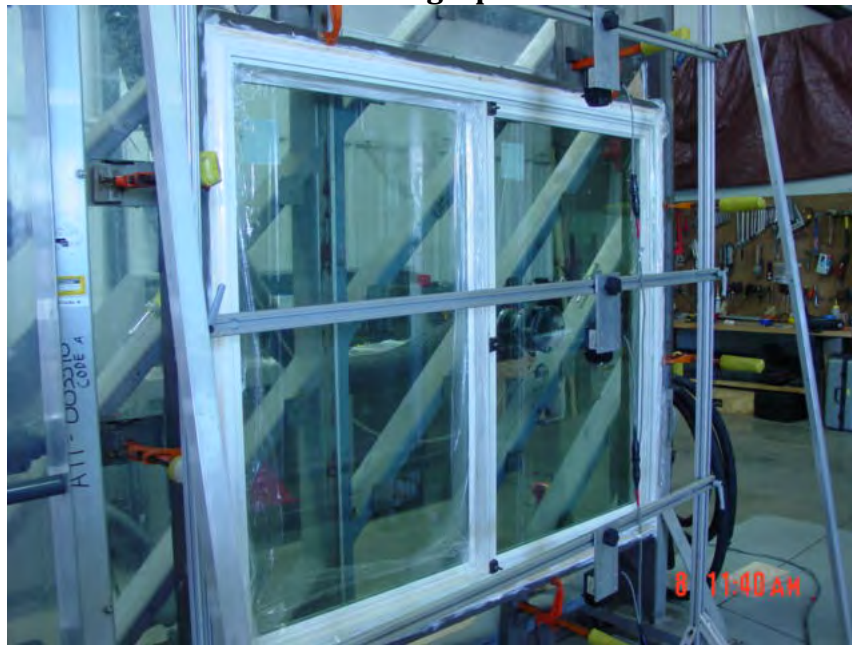
Photo #1 Structural loading on horizontal slider.
